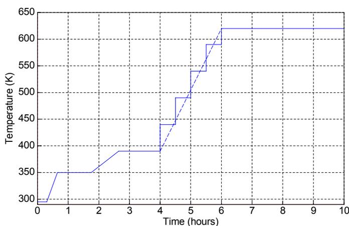
**Figure 2:** Recommended heating curve for the microporous material ERM<sup>®</sup>-FD107
