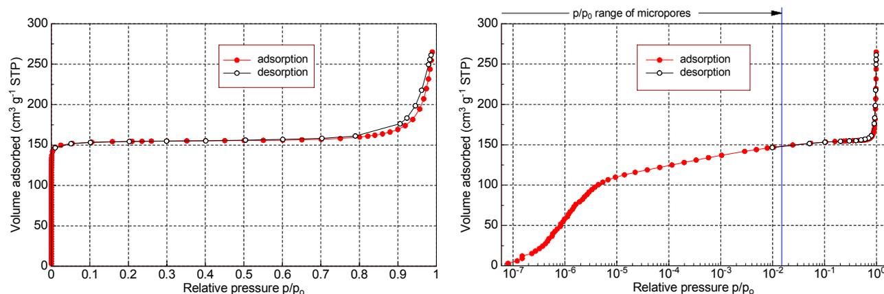
**Figure 1:** Linear and logarithmic plot of the nitrogen adsorption isotherm (non-certified) at 77.3 K and  $p/p_0$ -range for micropores (width  $\leq 2$  nm) according to the physical parameters applied in the Saito/Foley model with cylindrical pore geometry given on page 3.
